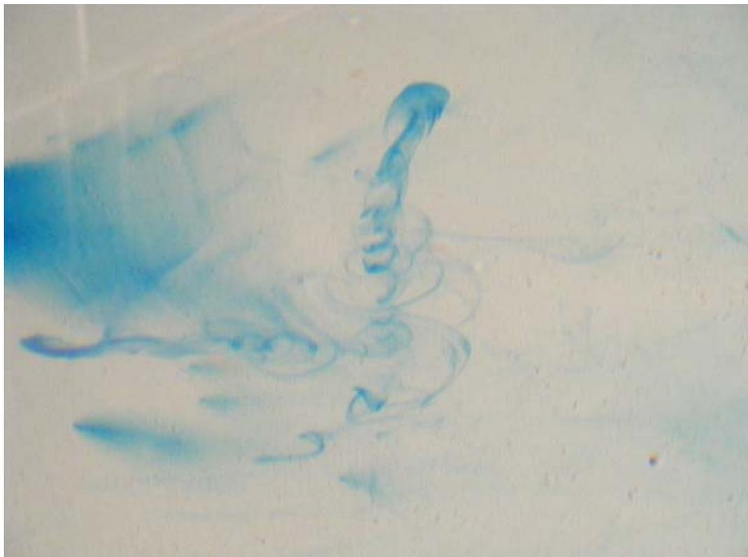
Figure 3: Photograph of a convective thermal plume rising from the bottom of the tank, visualized by blue dye. The plume is the core of a cyclonically circulating vortex of diameter  $\sim 10\text{-}20$  cm and around 30 cm high.
